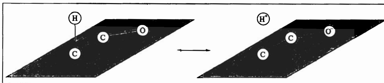
Fig. 4.14: Valence bond representation of the hyperconjugation effect which leads to a lengthening of the C-H bond in acetaldehyde.
