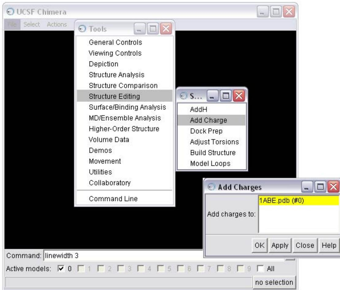
(B) To seed the charge calculation, Chimera needs the formal charge of the molecule. Chimera will estimate the value based on the atom types and bonding. Here, Chimera has estimated accurately, so we will calculate AM1BCC charges.
