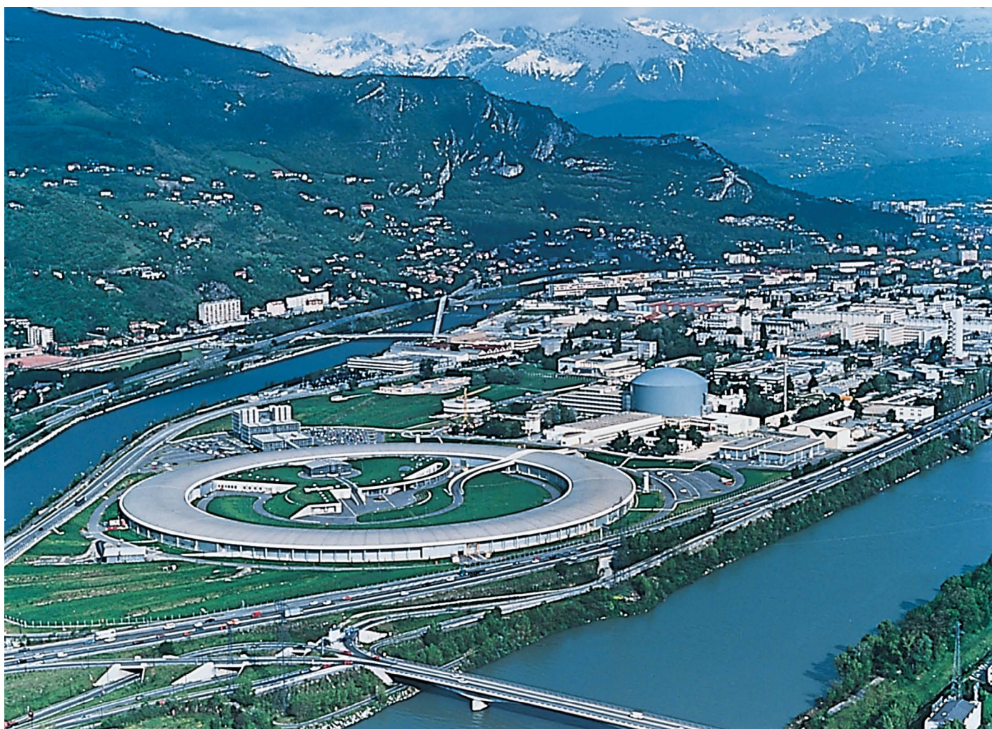
An aerial view of the European Synchrotron Radiation Facility at Grenoble, France, an advanced source of synchrotron x-ray radiation for use in the study of protein structure, as well as for use in the physical and material sciences. The synchrotron radiation is produced in the circular building in the lower left of the photograph. (Courtesy of ESRF.)
